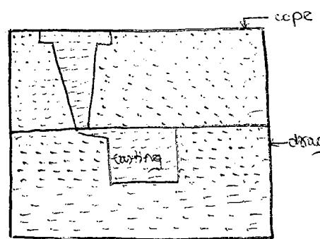
We pour the liquid molten metal in the casting cavity.
