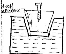
without providing draft allowance - until the last point of the pattern comes out from the mould , there is a contact b/w the pattern and the mould . and any shaking or vibration taken place to the hand make causes to damage the mould walls.
