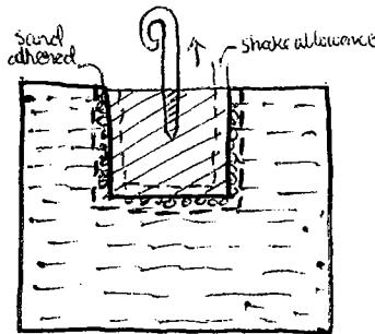
During removal of the pattern from the mould, whatever the moulding sand which has adhered to the pattern also gets removed and it damages the mould walls.
